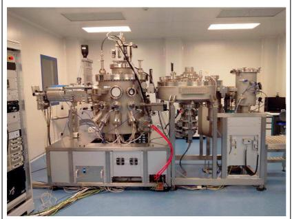
A silicon-germanium MBE equipment (SG800 from DCA Instruments) was recently installed at NanoTecMat technological platform. This MBE chamber is designed for 200mm wafer size. It is connected to a cluster tool type UHV central distribution chamber allowing future expansion with additional growth chambers, analysis chambers or other processing chambers.
