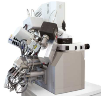
DualBeam : FEG with immersion lens + FIB (Gallium)
