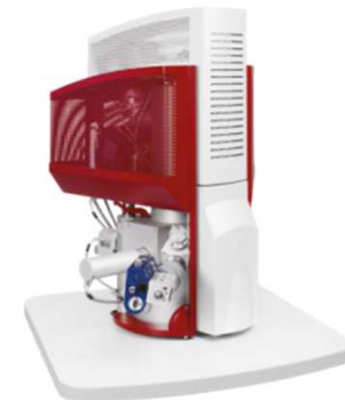
MEB FEG with immersion lens (ultra-high resolution for low-kV)
